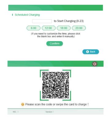
After swiping the card, the interface displays that charging is being scheduled, please do not unplug the gun. As shown in the figure; charging will automatically start at the scheduled time.
